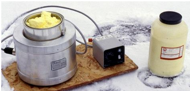
Fig. 10-16 Heating mantle with one-gallon unlined paint can.
