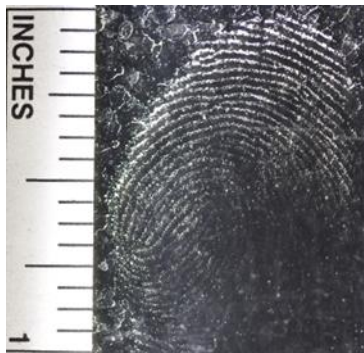
Fig. 11-4 Measurement increments should be visible in the photo to show whether they are in mm, cm, or inches.
