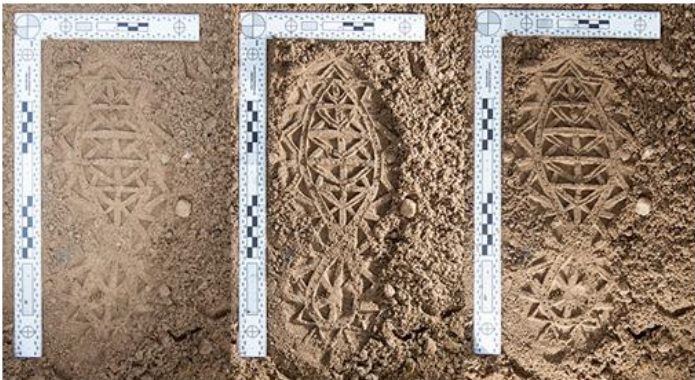
Fig. 3-7 These three photographs show the effect of the direction of light on the appearance of the details in a footwear impression. All three photographs are of the same footwear impression. The photograph on the left was taken with the flash on camera and is limited in pattern detail due to the lack of shadows. The center photograph was taken with the flash placed at a low angle on the right side of the impression. The right photograph was taken with the flash at a low angle at the bottom of the impression.
