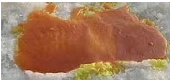
Fig. 10-19 Sulfur cast which has begun to harden.
