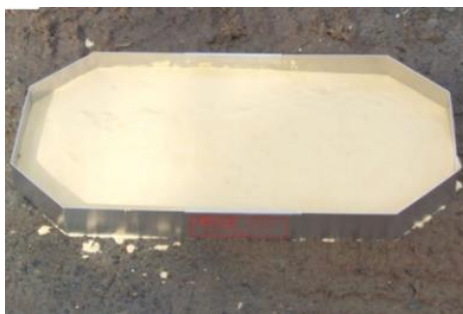
Fig. 10-13 Casting form placed around a submerged impression.
