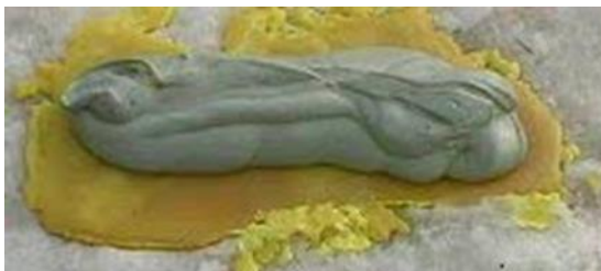
Fig. 10-20 Sulfur cast with dental stone reinforcement.
