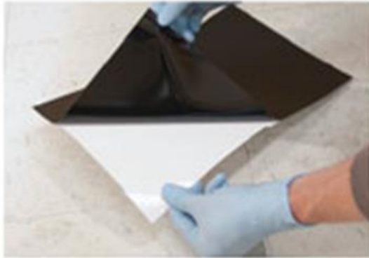
Fig. 10-5 Removal of backing paper from Stat-Lift™.
