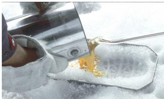
Fig. 10-18 Sulfur mixture is poured into the footwear impression using a deflector (metal spoon).
