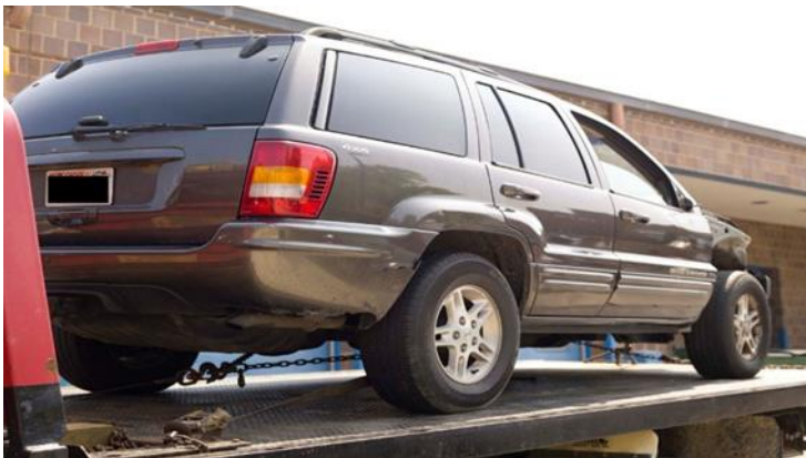
Fig. 22-2 Vehicle towed from undamaged end to an area laboratory.
