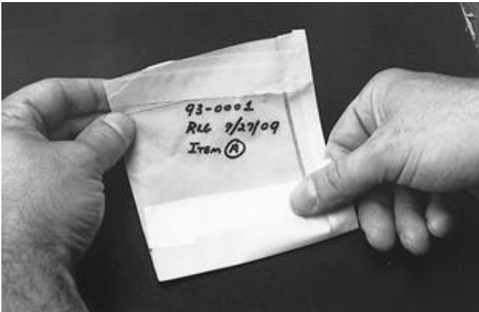
Fig. 17-4 Packaging Paint Sample: Carefully remove the paper from the object and fold each edge toward the center so that the packet is completely closed.
