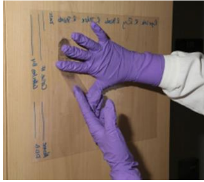
Fig. 11-22 Tape lifted from a finger is placed on the acetate sheet under the correct finger name on the opposite side of the writing.
