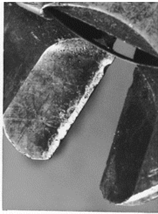
Fig. 16-4 Damage to the cutting edges of the blades creates individual markings on the materials cut by the bolt cutters.
