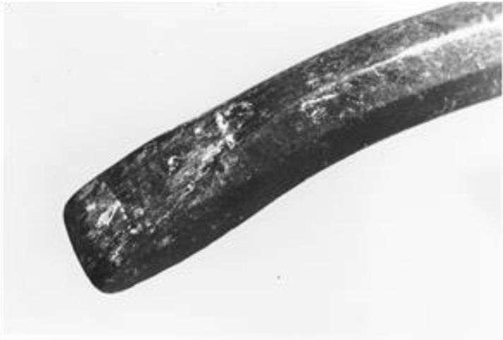
Fig. 14-1 Trace transfer of materials may be found adhering to pry bars.
