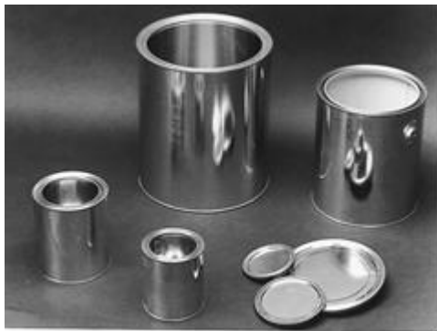
Fig. 25-1 New, clean paint cans make ideal containers for preserving evidence suspected of containing
