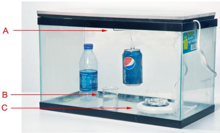
Fig. 11-2 Example of a typical superglue fuming chamber. (A) is a piece of wire from which items can be
