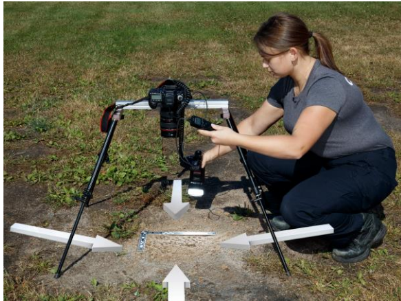
Fig. 3-8 It is recommended that a minimum of four images be captured of impressions, each lit from a different angle as illustrated above. Additional images lit from additional angles are beneficial.
