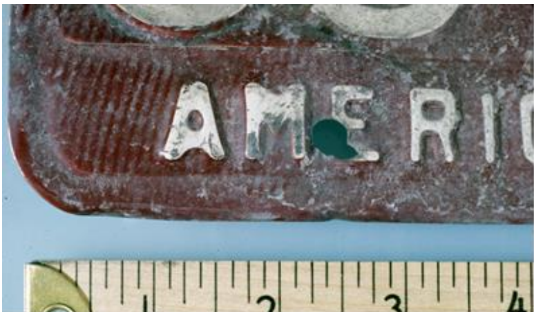
Fig. 19-1 Fabric impression on a license plate from a hit-and-run investigation.
