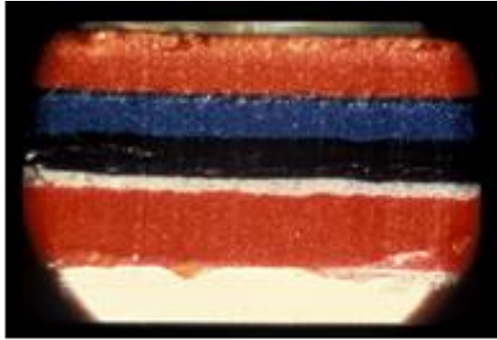
Fig. 17-2 Cross section of multi-layer paint chip. Each layer represents a separate painting operation (Magnification approximately X350).
