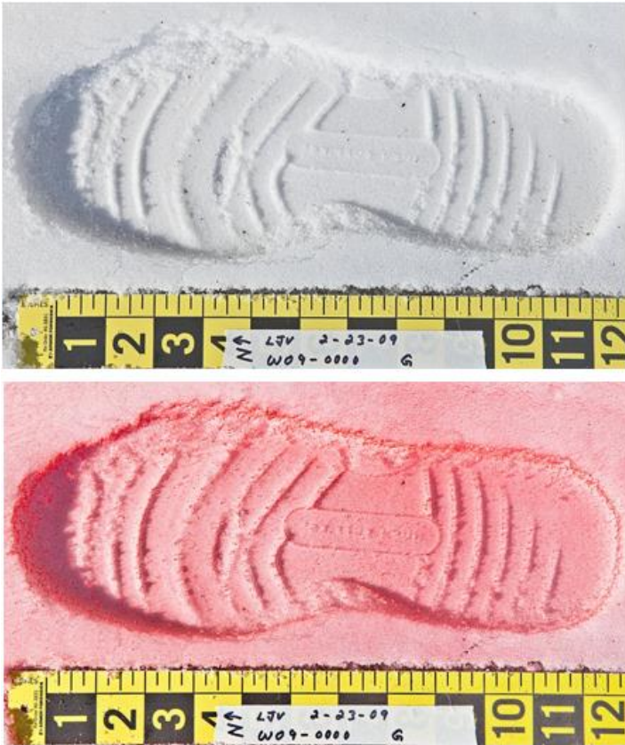
Fig. 10-15 Impression sprayed with Snow Print Wax™ which enhances the detail of impression and creates a buffer for the dental stone.
