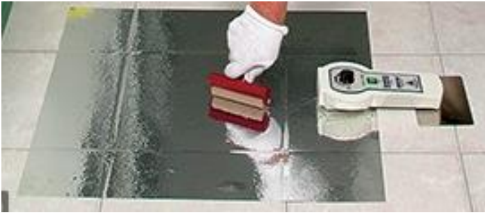
Fig. 10-3 Proper placement of electrostatic lifting device.
