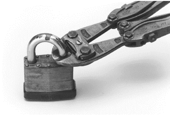
Fig. 16-3 Double-bladed tools such as bolt cutters are often used to cut padlock shackles. When recovered in the possession of a suspect, they may connect the offender with the crime.
