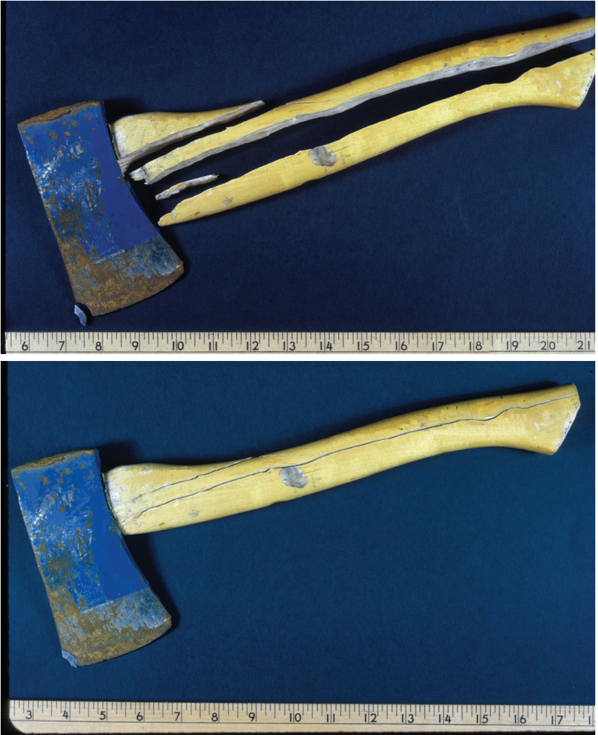
Fig. 22-2 Fracture match of an axe blade and handle.
