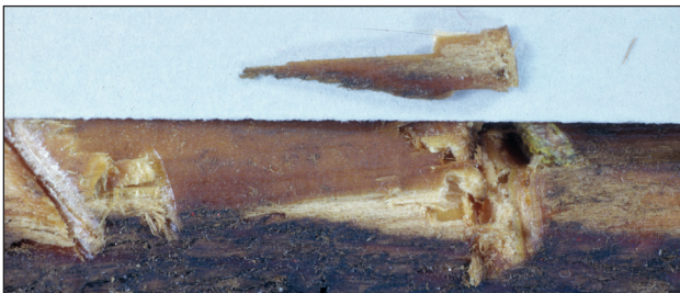
Fig. 22-1 Fracture match of a wood fragment to a piece of wood used as a bludgeon.
